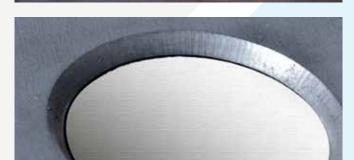
The 5-axis laser chamfer head enables Göcke to manufacture complicated contours and chamfers up to 52°, thus providing optimal conditions for subsequent welding processes. The smooth, burr-free cut edges of the blanks provide optimal conditions for flawless subsequent welding processes.
