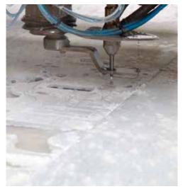
High pressure water jet cutting is a complementary process to the traditional, mechanical and thermal procedures. As no heat is applied for water jet cutting, steel, aluminum, non-ferrous metal, stone, glass, plastics, or sealing materials can be processed without problems.
